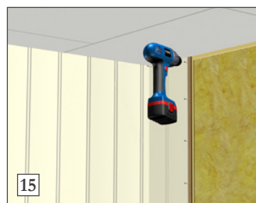
15) The panel is screwed in the nail lip. In the corner, the panel is fixed with dive pins (by hand). Secure top and bottom as usual. Use correction paint (in correct colour) to cover the visible screws.
